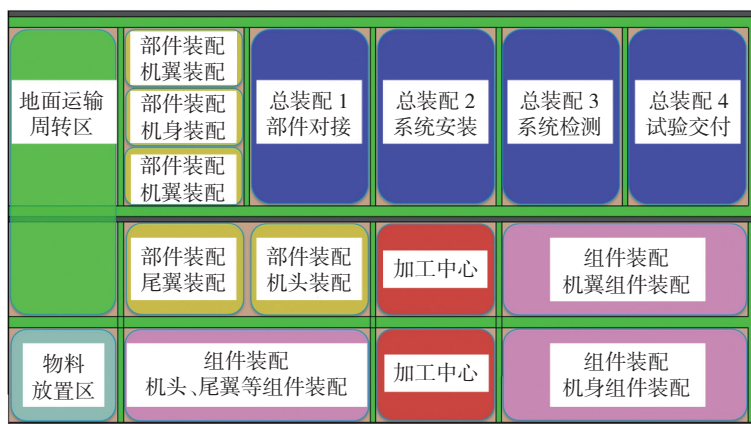
图7 厂房模块化规划 Fig.7 Plant modular planning
